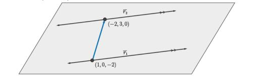
To obtain a second non-collinear vector in the plane, we determine the vector between the two given points on the lines; this is the vector (-2, 3, 0) - (1, 0, -2) = (-3, 3, 2).
